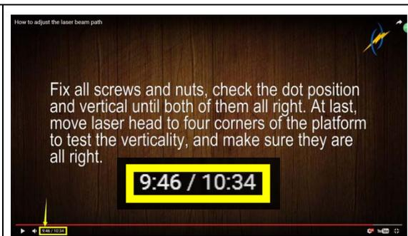
②When the laser head moves to four corners of the working table, check if the laser beam can vertically go through the 10mm acrylic.
